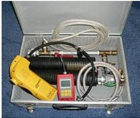
Duct Tightness Testing Kit
