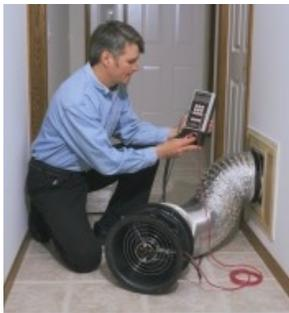
Testing the Duct Tightness
