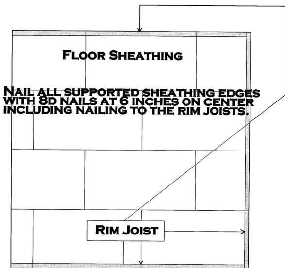
The International Residential Code, Table 602.3(1), specifies how wood structural panels need to be attached to other structural building components, such as walls, floor and roofs. When the floor sheathing is nailed down to the floor joists, all panel edges that are supported by framing (floor joists, rim joists and
